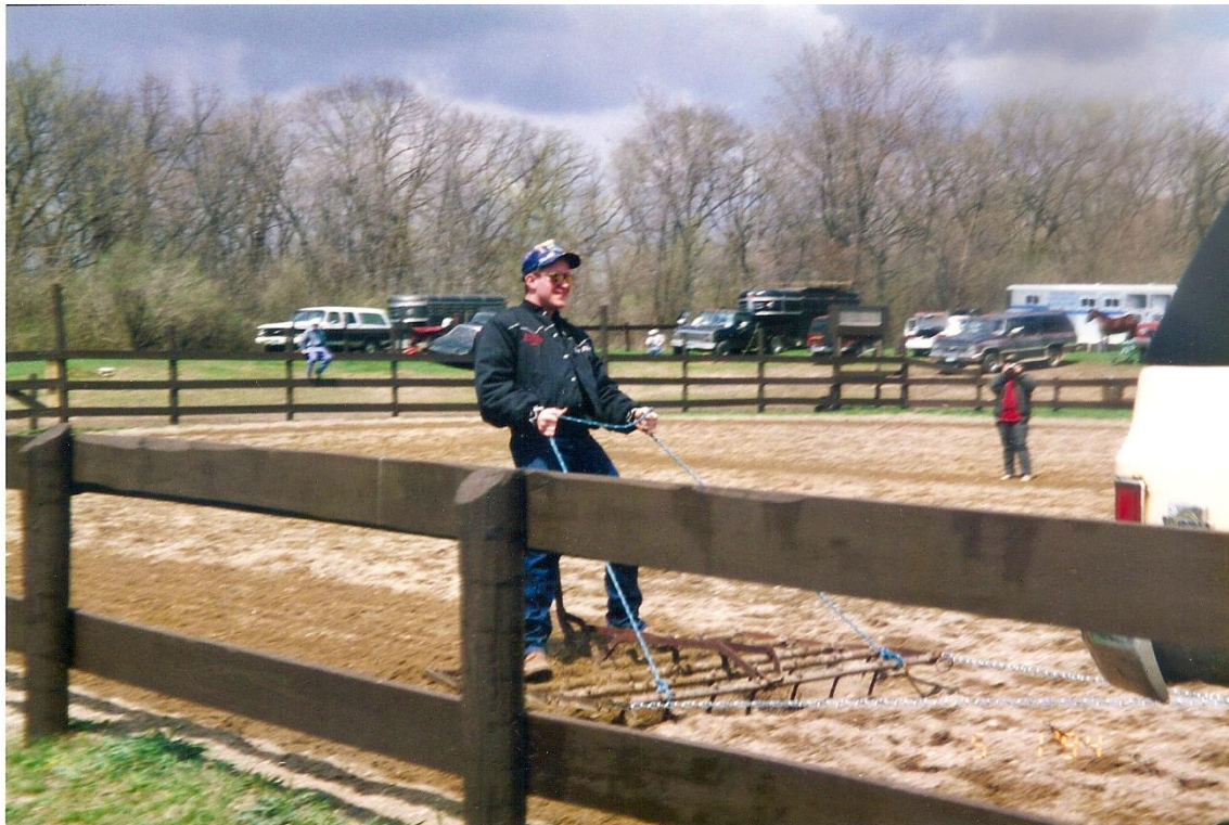
Figure 9 – Power raking the horse ring sand before a show in 1992. The person standing on the rake device is ballast to keep the rake from jumping as it was pulled.
